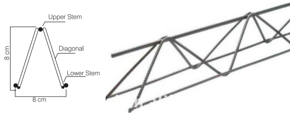
Figure 19. Example of lattice girder reinforcement
