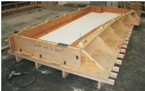
Figure 44. Custom made wooden mould
