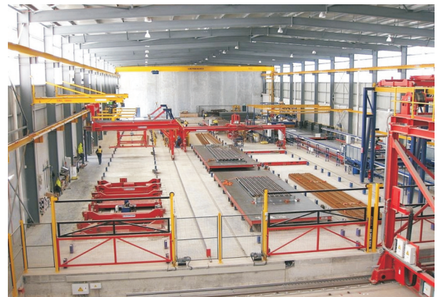
Figure 42. Circulating pallet system (flat moulds)
