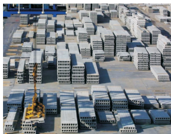
Figure 6. Mass production of standard slabs
