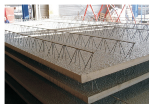
Figure 17. Precast half slab with lattice girders
