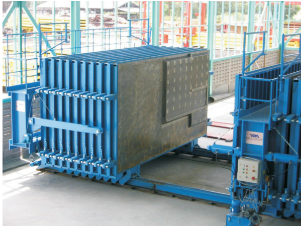
Figure 43. Battery mould (vertical moulds)
