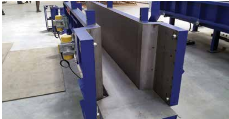
(Picture 26. Special stationary mould for precast columns)
