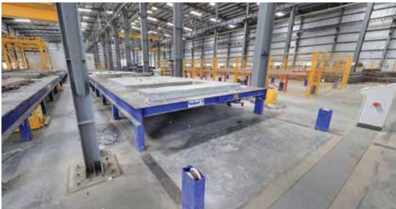
(Picture 24. Circulation system for horizontal production of precast wall panels and slabs)
