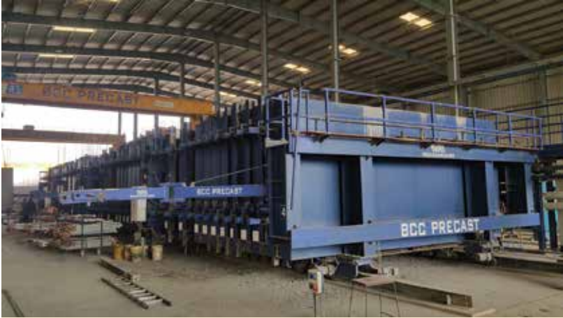
(Picture 10. Battery mould for vertical production of precast wall panels)
