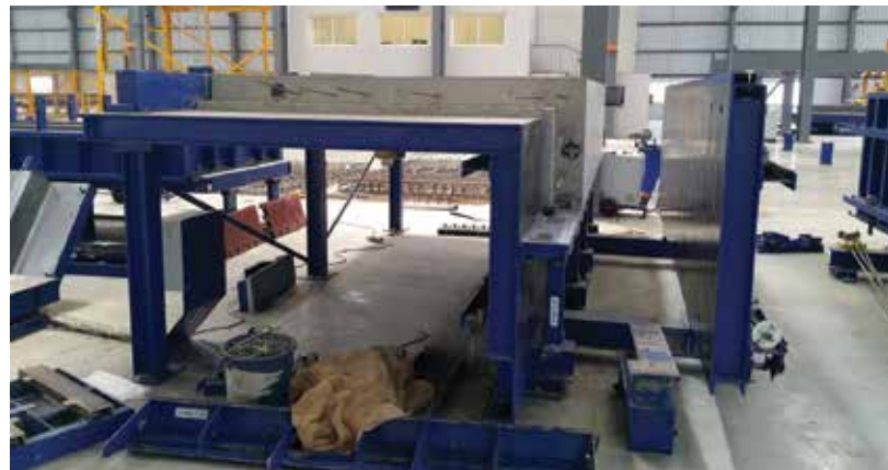
(Picture 25. Special stationary mould for L-shaped walls)
