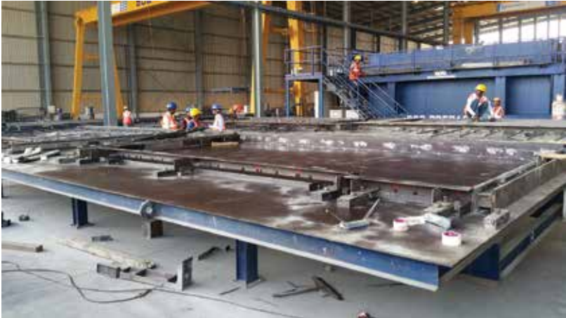
(Picture 12. Tilting tables for horizontal production of precast wall panels)
