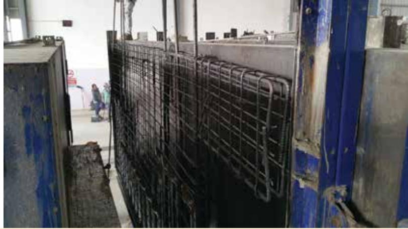
(Picture 11. Precast wall panel reinforcement cage inside battery mould system)
