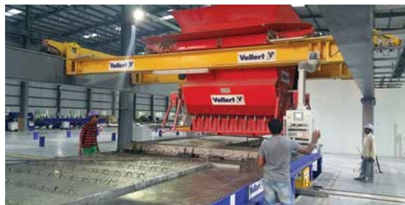
(Picture 28. Concrete spreader for pouring of concrete)
