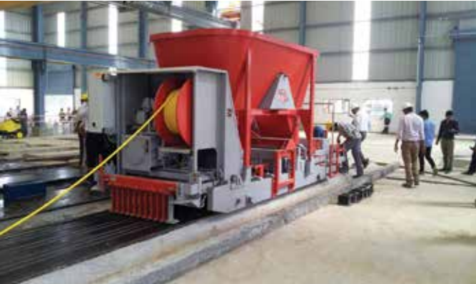
(Picture 38. Prestressed hollow core production with slipformer machine)
