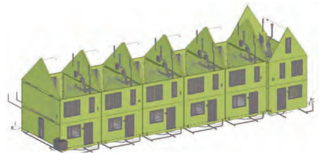
Fig. 8: Precast Structure 3D Model with Integrated MEP Services
